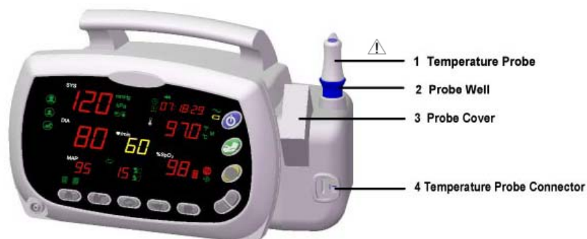
Figure 6. Temperature Probe Connections
